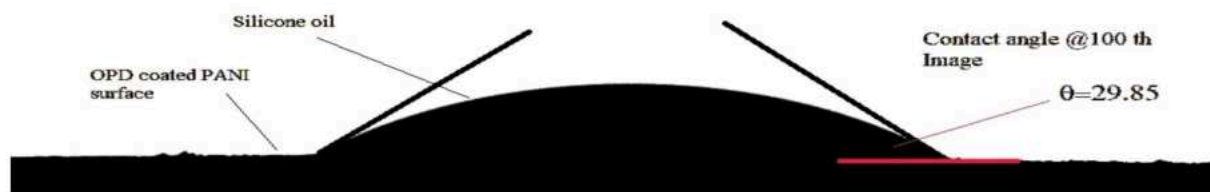
Figure 25: Contact angle measured on OPD coated PANI surface-100th image.
