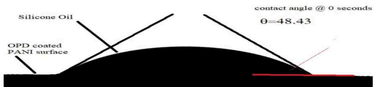
Figure 24: Contact angle measured on OPD coated PANI surface-1st image at 0 seconds time image .
