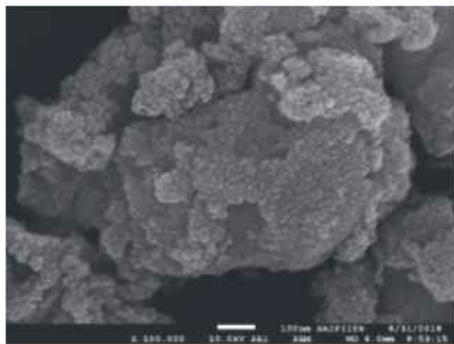
Fig. 2: FEG- SEM image of Mn 0.8 Co 0.2 Fe 2 O 4 spinel ferrite nanoparticles
